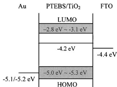
FIG. 9. Flatband energy diagram for the devices of FTO/TiO<sub>2</sub>:PTEBS/Au.
