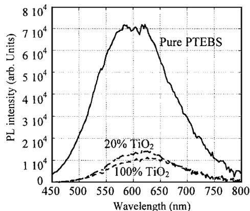
FIG. 5. The photoluminescence spectra from PTEBS:TiO<sub>2</sub> films for 0%, 20%, and 100% TiO<sub>2</sub>.
