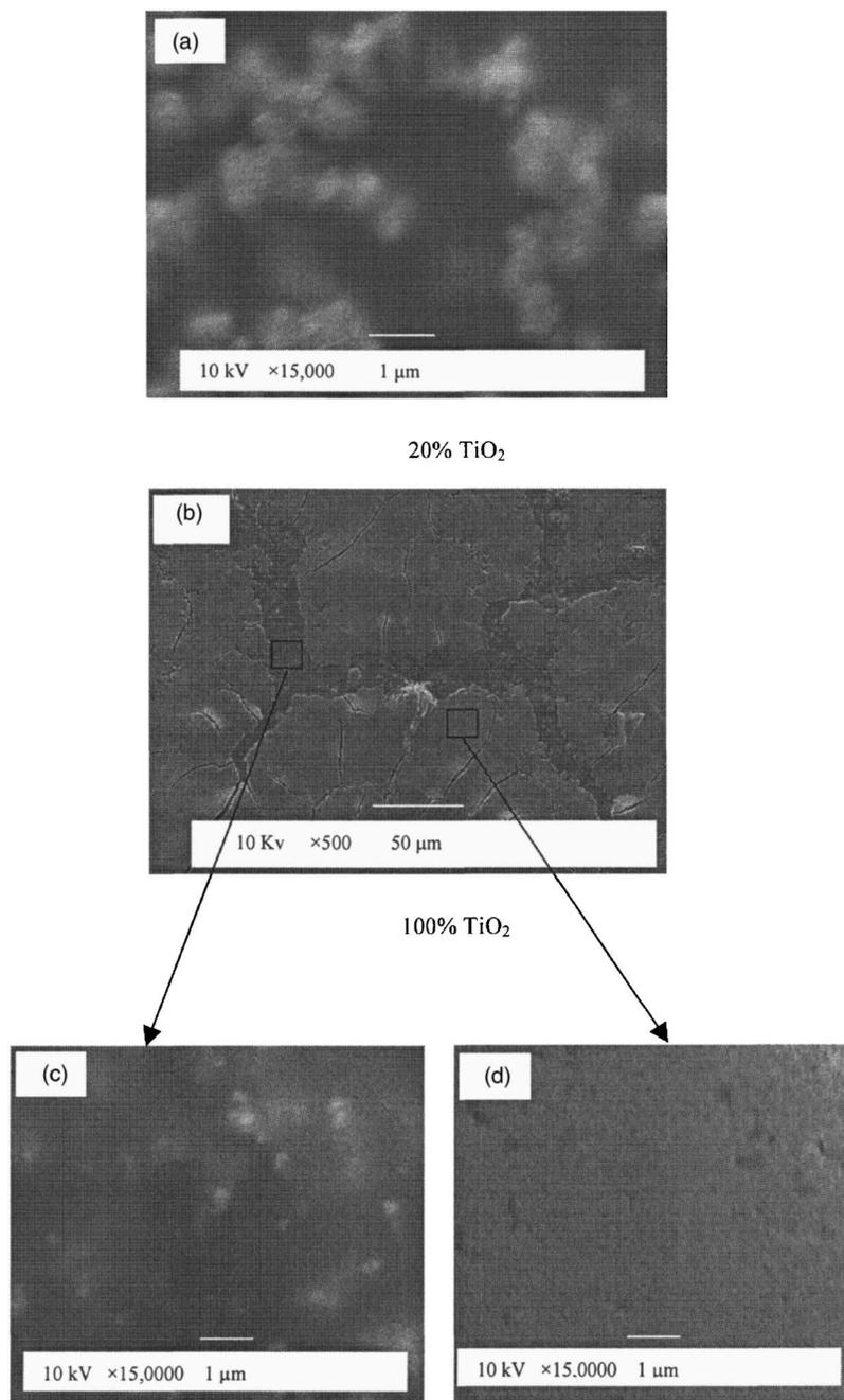
FIG. 6. SEM images of films from (a) PTEBS:TiO<sub>2</sub> (1:0.2), (b) PTEBS:TiO<sub>2</sub> (1:1), and [(c) and (d)] amplified SEM for PTEBS:TiO<sub>2</sub> (1:1).
