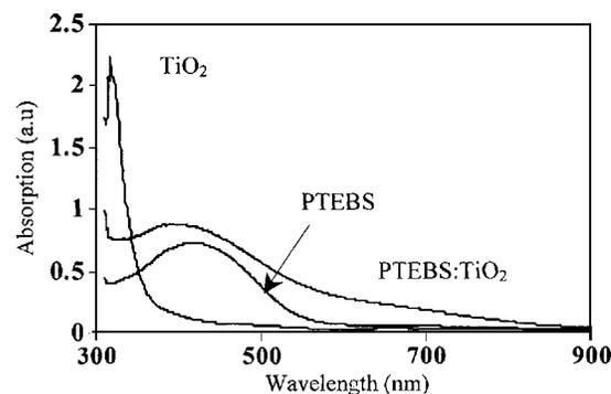
FIG. 2. Absorption spectra of PTEBS, TiO<sub>2</sub>, and 1:1 (by weight) PTEBS:TiO<sub>2</sub> composites on a FTO glass substrate.
