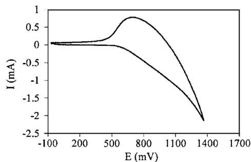
FIG. 4. Cyclic voltammogram (ref. SCE) of cast thin film of PTEBS on FTO substrate in CH<sub>3</sub>CN/LiClO<sub>4</sub> 0.1M.
